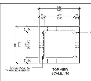
\* BOLTING PATTERN DESIGNED TO MOUNT PEDESTAL SOLUTIONS INC. SLM MODELS
