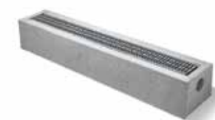
Driveway Catch Basin 300mm x 410mm x 1,980mm (12" x 16" x 78"); comes with grate and 100mm (4") drain holes
