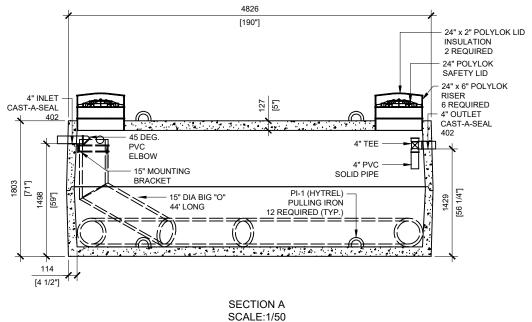
2540 [100"] 24" x 2" POLYLOK LID INSULATION 2 REQUIRED 24" POLYLOK SAFETY LID 24" x 6" POLYLOK 127 [5"] RISER 6 REQUIRED 45 DEG. PVC ELBOW 15" MOUNTING\_ [4"] **BRACKET** [61"] [71"] 15" DIA BIG "O 44' LONG 127 [5"]
